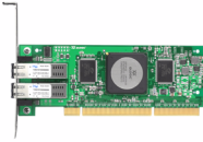
64-bit PCI-X 2.0 connector
